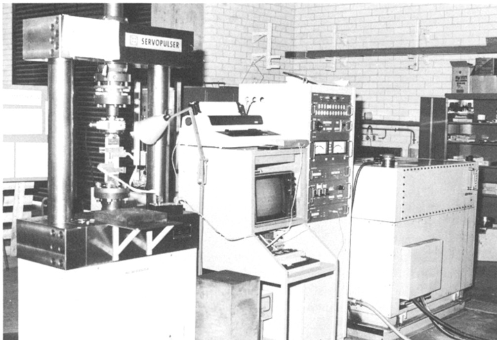
Figure 1 General view of hardware of the computerized crack monitoring system.
